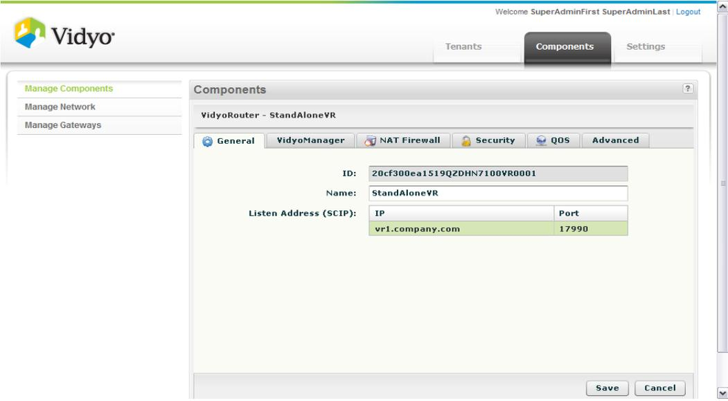
The screenshot shows the Vidyo web interface for configuring a StandAlone VidyoRouter. The 'Listen Address (SCIP)' section is highlighted, showing a table with the following data:
