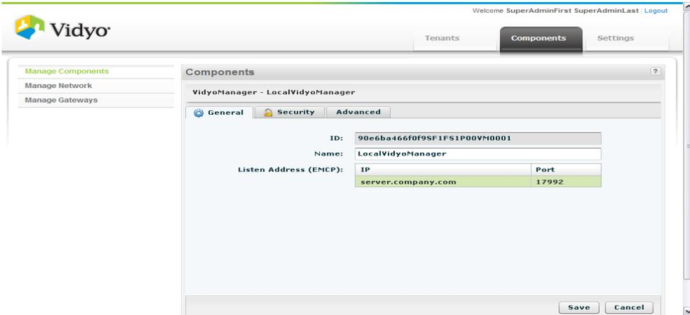
The screenshot shows the configuration page for the 'LocalVidyoManager' component. The 'Listen Address (EMCP)' section is highlighted, showing the following fields:
